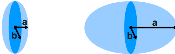
Figure 3: Oblate (left) and prolate (right) ellipsoid and the corresponding radii. The movement of ellipsoids in the fluid is from left to right.
